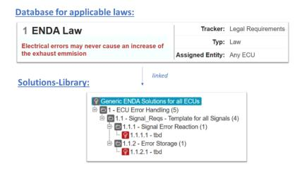
As depicted in the following diagram, a linked solution is e.g. a generic template for all signals, which secures that for each of the signals the Signal Error Reaction and the Error Storage are specified (to ensure that it is implemented and tested), without defining the details how this shall be performed (by using the placeholder *tbd*).
